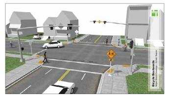
Where there are more than three lanes across, more robust crossing treatments may be necessary. One such treatment is the hybrid beacon. Hybrid Beacons can facilitate bicycle crossing of a busy street where cross traffic does not stop but motor vehicle traffic volumes on the calm street do not warrant a conventional traffic signal. The hybrid beacon flashes red lights to alert drivers on the cross street that bicyclists are present and intend to cross the street.
