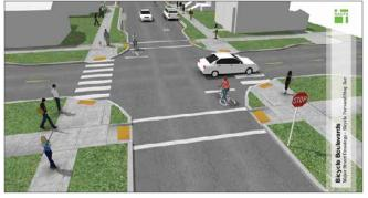
FIGURE 2.3.7.9: BICYCLE FORWARD STOP BAR
