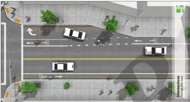
FIGURE 2.3.7.7: RIGHT TURN LANE WEAVING AREA
