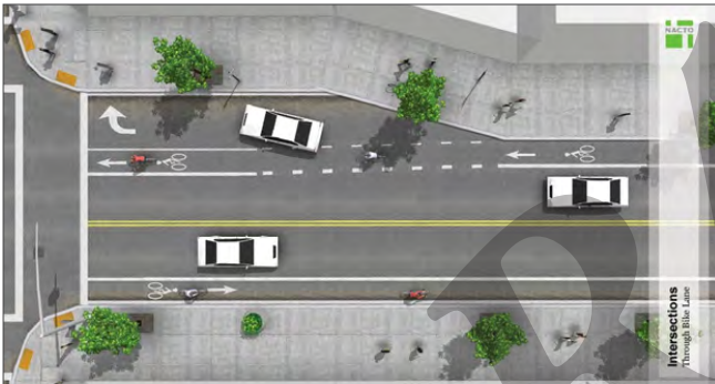
FIGURE 2.3.7.7: RIGHT TURN LANE WEAVING AREA
