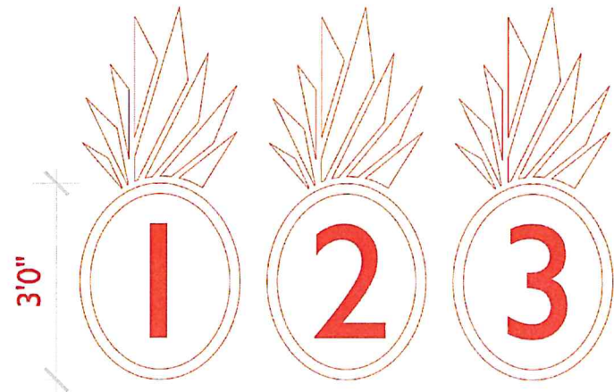
PICKUP PARKING PAVEMENT MARKING NO SCALE
