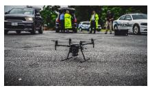
Since April 2019, the Florissant Police Department has utilized a state-of-the-art small Unmanned Aircraft System (sUAS) unit to enhance public safety and support law enforcement operations. The department operates two DJI Matrice 210 drones, equipped with advanced features such as a zoom lens camera, thermal imaging capabilities, LED flood/spotlights, and a payload drop
